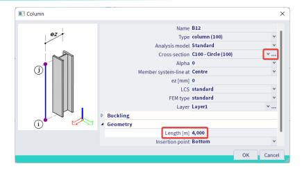
Define a circular cross section from this window, define a length of 4m and close the window by clicking on "OK". Now you can use the previous enabled snap settings to add 9 columns because the straight beam was now divided in 10 equal pieces to snap to.
