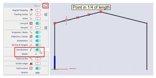
We are going to rotate the purlins so that their LCS Z-directions points in the same direction as the LCS of the frame beams.
