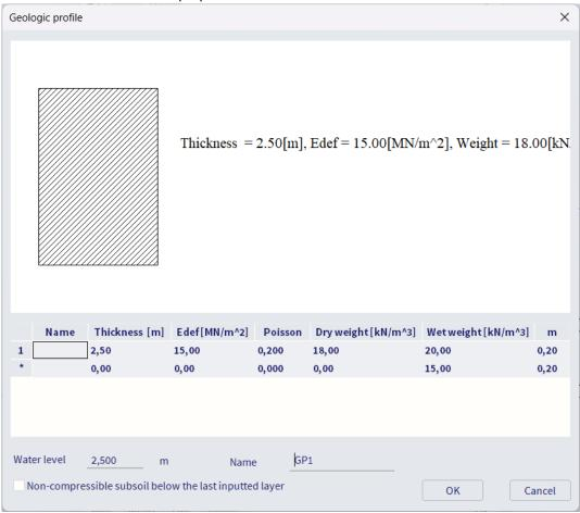
The top of the profile should represent the zero level of the ground, therefor input the borehole on top of the pool.
