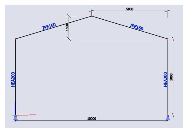
Insert the first frame of the hall as shown in example 2.
