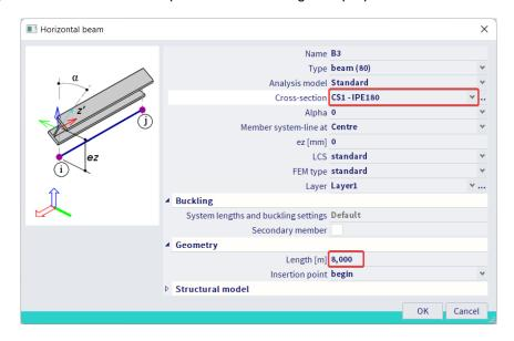
Click 'OK' to start modelling. The beam is entered from the beginning (left side) so again enter coordinates first '-2,5 3' and ESC to close the action.
