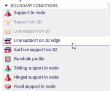
Set the restriction as sliding and click on the left and right 6m edge of the slab we just created to add the supports.
