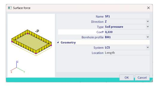
The coefficient can be used to define the active ground coefficient. Click on ok and select the walls of the pool that should be loaded with a horizontal ground load.
