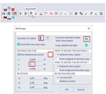
Because you enabled the upper right option right after you click 'OK' a new window appears to choose a cross section which is going to be applied to the additional members. Click on the manage option next to the cross section property and add another IPE 100 for the purlins.
