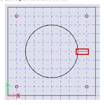
We are going to use multicopy to define the remaining part of the stiffners. But a rotational copy is always defined around the UCS sytem. So we are going to move it to the center of the column:
