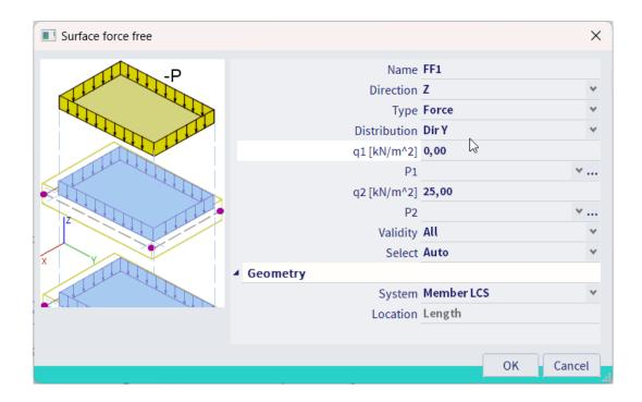
Draw a free surface and do so for UCS YZ as well as XZ to have loads in both directions:
