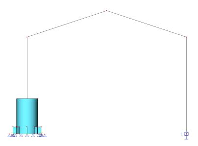
Filter the Input Panel category filter to "Boundary condition" and chose for "Line rigid link". Select the end node of the column and afterwards the upper edge of the detail:
