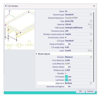
Draw a rectangular slab from coordinates "0 0 0" to "8 5 0", end with ESC and fill in the properties of the rib:
