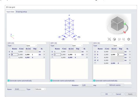
Click on "OK" and enter the grid in the origin so that the grid dimensions fall in line with the coordinates in Scia. Enter "0 0 0" in the SCIA spotlight. End with ESC.
