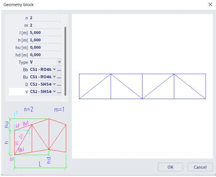
We are going to use the same cross section for the whole cross section. Close the windows with "OK" and enter the truss on coordinates 1 0 5.
