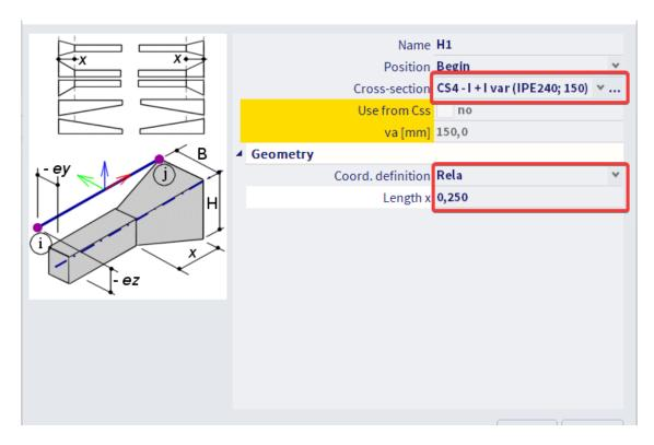
And click on the element where you want to add the haunch on, the beams of the frame in our case:
