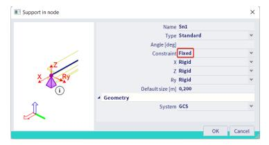
Simply select the nodes where you want these supports to be applied to and end action with ESC.
