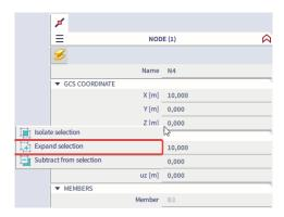
When you used one of the above methods to select the correct node you can add a hinged support by filtering the category of the Input Panel to 'Boundary conditions' and choosing 'Hinged support in node':
