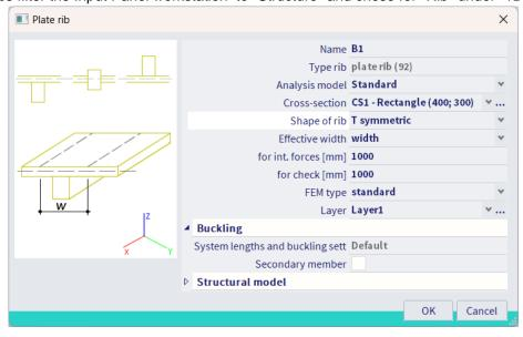
Then simply draw the ribs onto the slab using the following coordinates: " $0\,0.5\,0$ "-" $8\,0.5\,0$ ", " $0\,1.5\,0$ "-" $8\,1.5\,0$ ", " $0\,2.5\,0$ "-" $8\,2.5\,0$ ", " $0\,3.5\,0$ "-" $8\,3.5\,0$ ", " $0\,4.5\,0$ "-" $8\,4.5\,0$ ".
