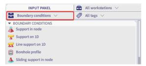
Change the properties in the next window as shown below and select the nodes where you want to apply the support to, bottom two nodes for this example.
