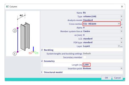
Click 'OK' and draw the left column by entering '0 0' and clicking ENTER to end the action. You can now click ESC to close the action or enter another coordinate: enter '3 0' for the right column, click enter and close the action with ESC. Note that coordinates are separated with a SPACE in between them. Because we are in a 2D environment, we only need to fill in 2 coordinates.
